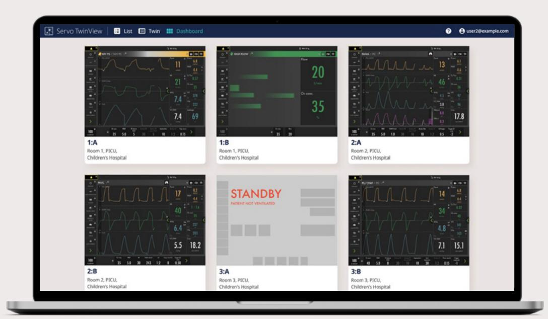
The Dashboard View displays up to six ventilators simultaneously, offering a comprehensive patient view and facilitating easy switching between different beds. The location is shown for each ventilator system, and the filters set in the List View also apply to the dashboard.
