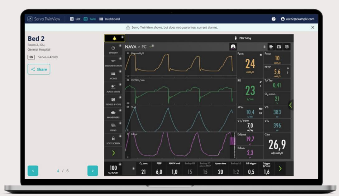
The Twin View presents a near-real-time twin of the user interface of the selected ventilator system. Users can access functions to view basic numerical values, current alarms, and other information, providing an enhanced understanding of the patient's status.
